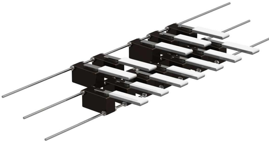
Figure 11.1: A concept draft of the keyboard module design created in *NX 4.0*.
