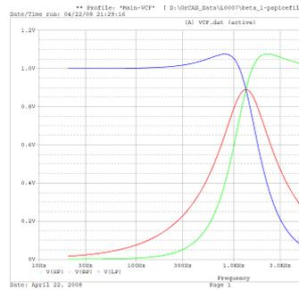
Figure 7.3: Simulated frequency response plot of the voltage controlled filter with 50 % resonance and control voltage of  $1\text{ V}$ . The cutoff potentiometer is held at  $50\text{ k}\Omega$
