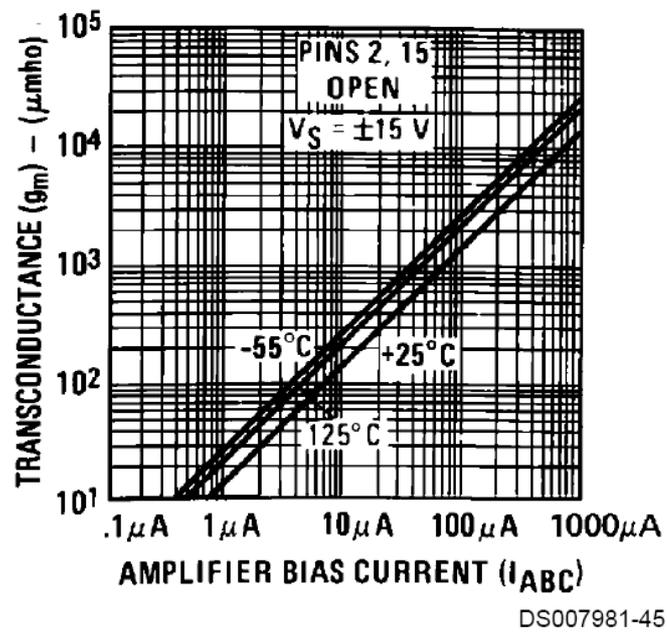
Figure C.1: Transconductance of the *LM13700*
