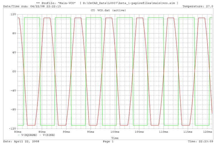
Figure 8.4: A simulated output of the voltage controlled oscillator with 12 V control voltage
