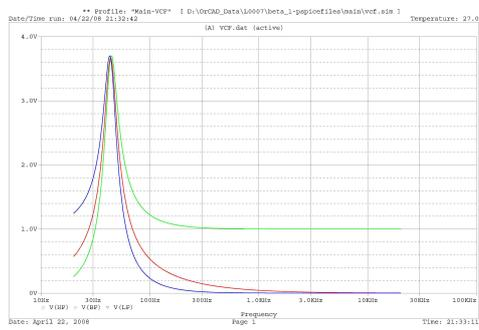
Figure 7.5: Simulated Bode-plot of the Voltage Controlled Filter with 100 % resonance and 0 % cutoff and 1 V control voltage
