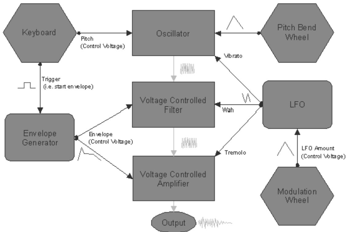
Figure A.1: Practical correlation between different parts of an analog synthesizer, [1]
