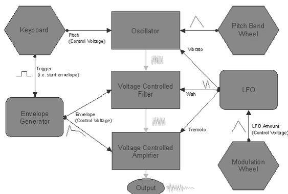
Figure 3.1: Practical correlation between different parts of an analog synthesizer, [1]. An enlargement can be found at page 59.
