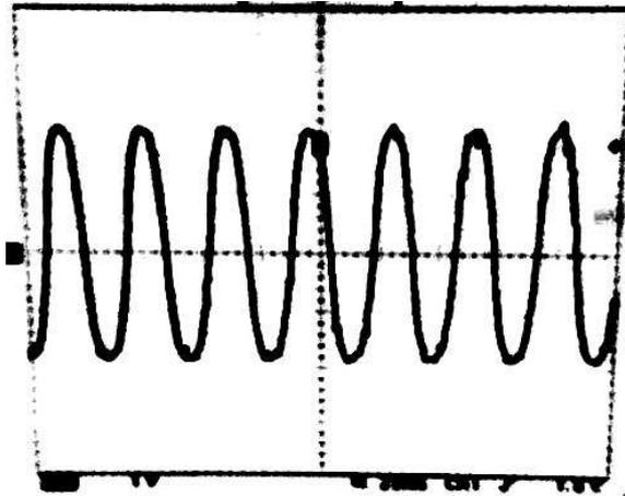
Figure 14.5: Low Frequency Oscillator sine wave output at about 30 Hz
