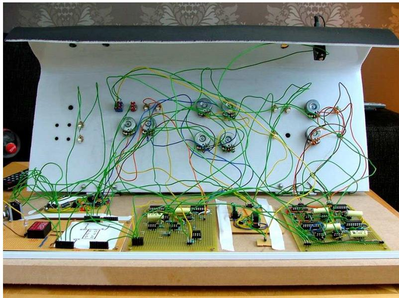
Figure 13.1: Interconnection of the Power Supply Unit, Voltage Controlled Filter, Attack-Release Envelope generator and the Voltage Controlled Oscillator. On the top left there is the Low Frequency Oscillator, control potentiometers and more
