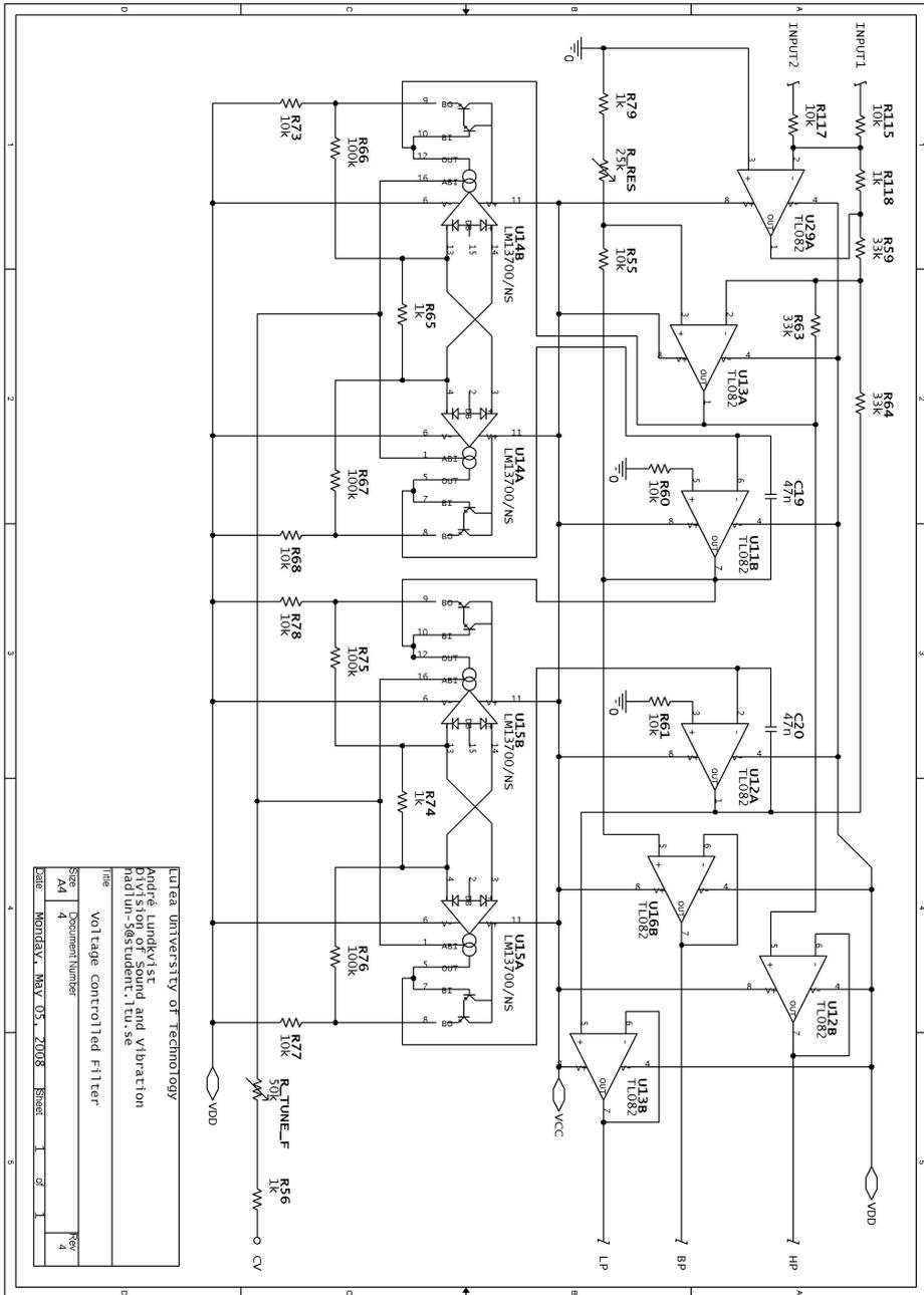
Figure D.3: Final circuit design of the voltage controlled filter
