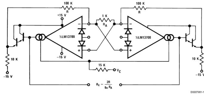
Figure 7.2: Floating point voltage controlled resistance, [7]
