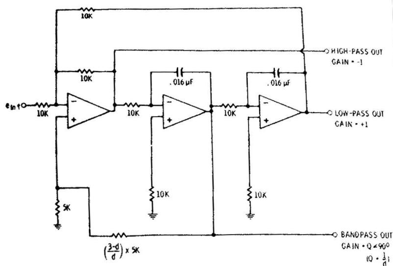
Figure 7.1: A unity gain, state-variable filter [3]
