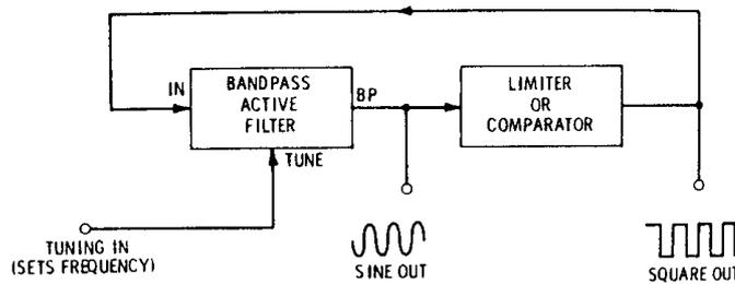
Figure 8.1: A way of creating a voltage controlled oscillator based on an active bandpass filter. [3]
