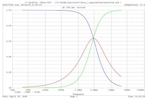
Figure 7.4: Simulated Bode-plot of the Voltage Controlled Filter with resonance at 0 % and a cutoff at 100 % and 1 V control voltage
