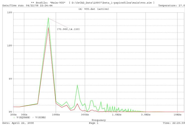
Figure 8.3: A *Fast Fourier Transform* analysis of the simulated output of the voltage controlled oscillator with 1 V control voltage. Ground frequency is 75 Hz
