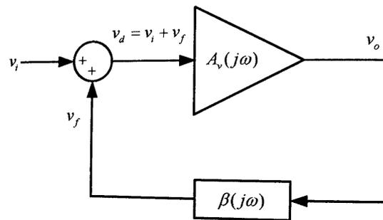
Figure 2.1: A simple feedback oscillator circuit [4]
