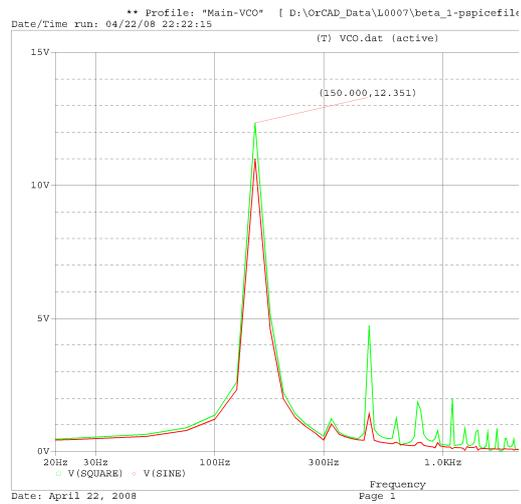
Figure 8.5: A *Fast Fourier Transform* analysis of the simulated output of the voltage controlled oscillator with 12 V control voltage. Ground frequency is 150 Hz
