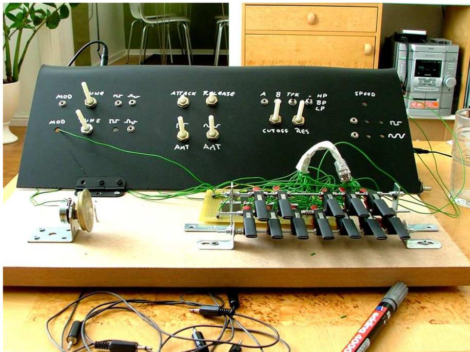
Figure 12.2: The mounted body with control potentiometers, keyboard module and bend wheel
