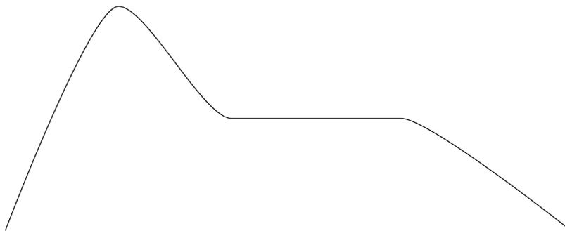
Figure 10.1: A control voltage envelope of a classical ADSR envelope generator
