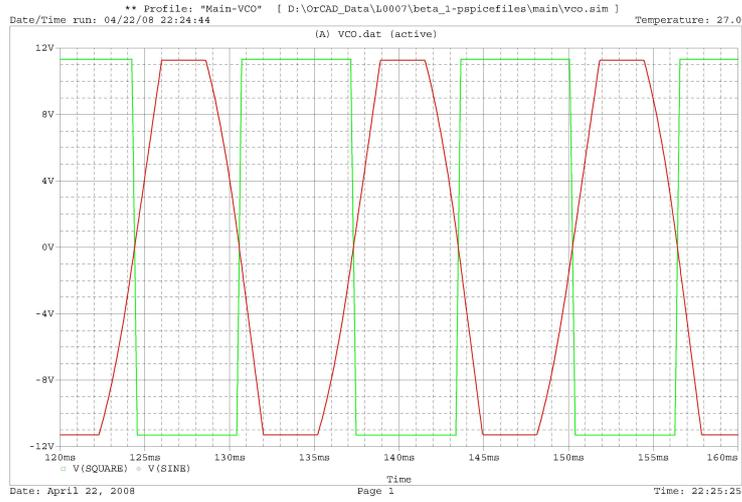
Figure 8.2: A simulated output of the voltage controlled oscillator with 1 V control voltage
